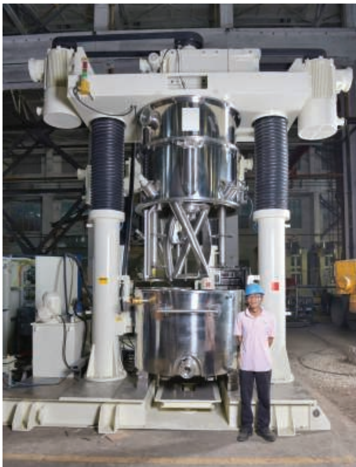
FIGURE 2. The agitators in this 300-gal planetary disperser are lifted out of the vessel via a dual-post hydraulic lift, allowing complete access for cleaning and maintenance
