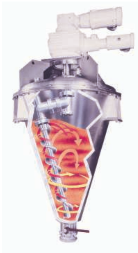
FIGURE 6. The agitator movement and material flow pattern shown here for a vertical blender-dryer provides favorable results for many applications. Product is heated through contact with the jacketed sidewalls. The vacuum-rated cover may also be jacketed to avoid condensation
