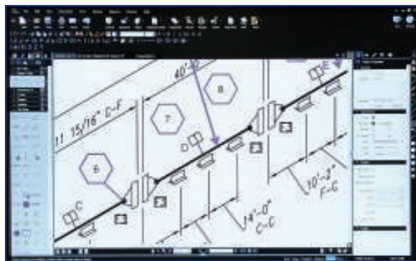
McCarl's uses the Sequence Tool in Revu to number and track all of the welds that need to be made in the fabrication shop
