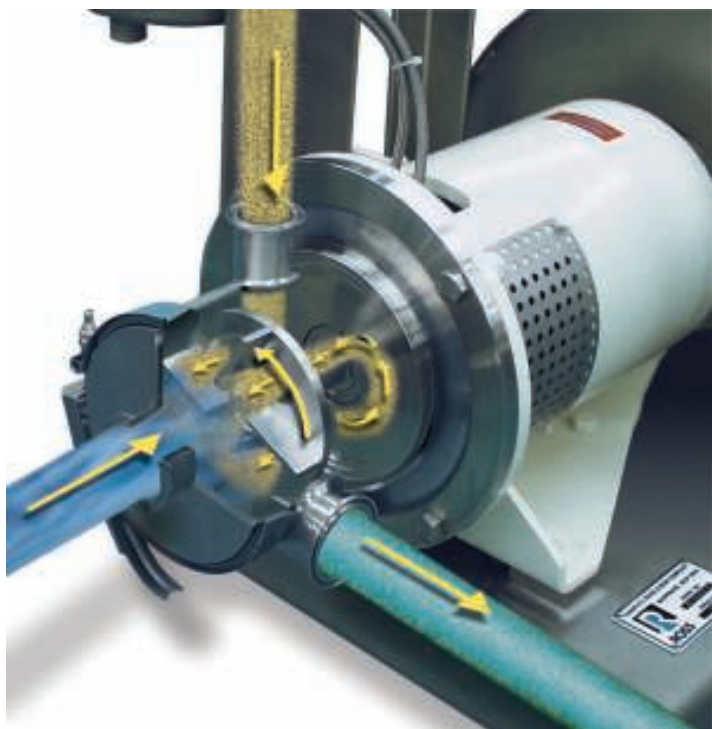
FIGURE 3. This illustration shows how a powder-induction mixer works. The liquid stream (blue) enters the mixer and immediately encounters the powder addition. Drawn by a powerful vacuum, free-flowing powders (yellow) are injected into the liquid and instantaneously mixed under high shear. The resulting dispersion (green) is expelled centrifugally through the stator openings at high velocity
