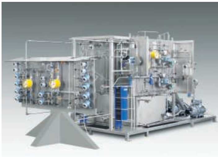
FIGURE 9. Shown here is a forced-circulation system serving several mechanical seals
