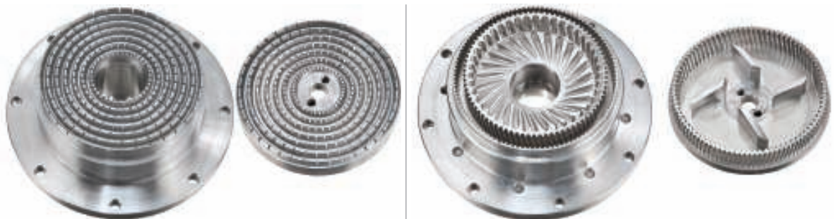
FIGURE 5 (below). Shown here are some examples of the rotor-stators used in modern ultra-high shear mixers. The combination of high tip speed and extremely close tolerances between the interlocking channels subjects the product to intense shear in a single pass. The gap between adjacent surfaces of the rotor and stator is adjustable, allowing operators to fine-tune shear levels and flowrates
