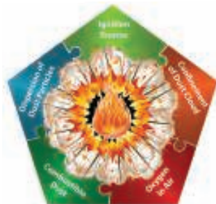
The combustible dust pentagon: removal of any one element can prevent explosions
